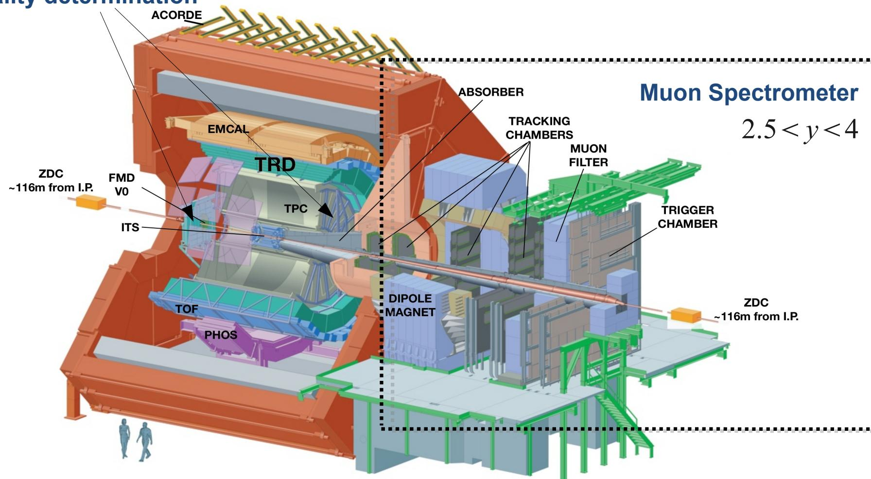
Dimuon trigger provided by the coincidence of two single muon trigger signals with a  $p_{T,\mu}$  threshold at about 0.5 GeV/c (pp) or 1 GeV/c (Pb-Pb)
