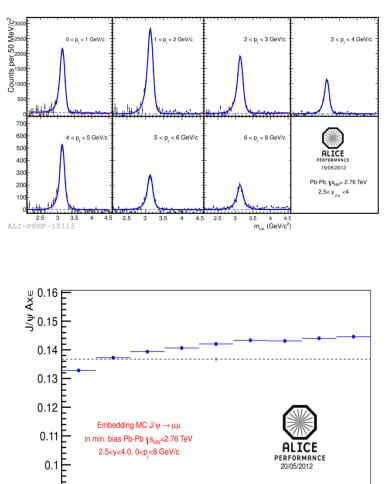
Yield extracted by fitting the invariant mass spectrum of unlike-sign dimuons:
