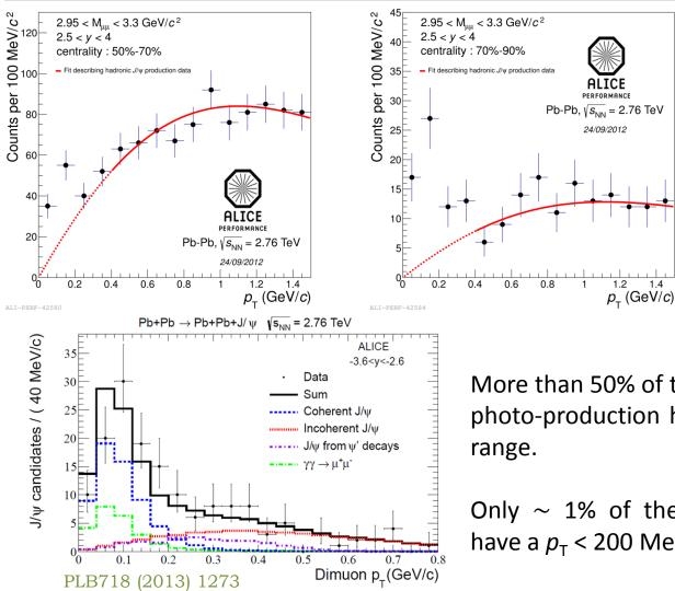
Clear deviation, at low-  $p_T$  for semi and peripheral collisions, to the expected J/ $\psi$  hadro-production.
