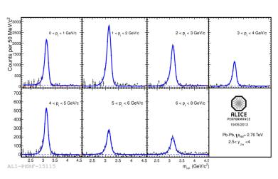
Yield extracted by fitting the invariant mass spectrum of unlike-sign dimuons:
