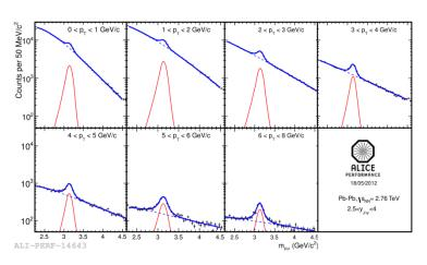
Yield extracted by fitting the invariant mass spectrum of unlike-sign dimuons:
