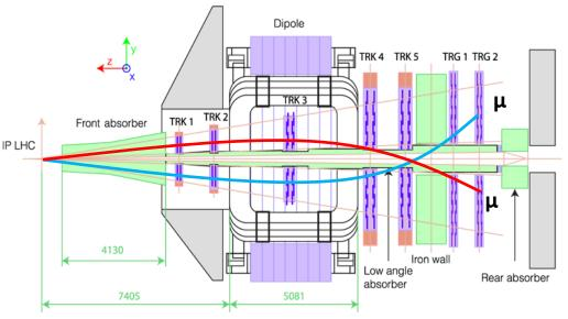
• Tracking chambers.- Spatial resolution, in bending coordinate, better than 100  $\mu$ m in order to identify and disentangle the  $\Upsilon$  family (100 MeV resolution).
