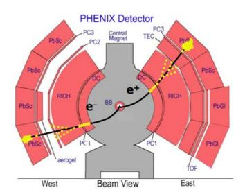
Energy in calorimeter electron ID in RICH Tracking in Drift chamber
