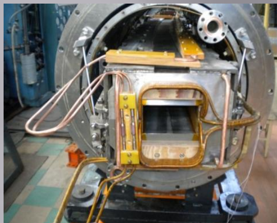
Dipole magnet in cryostat
