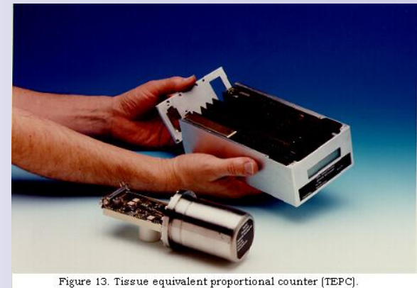
Figure 13. Tissue equivalent proportional counter [TEPC].
