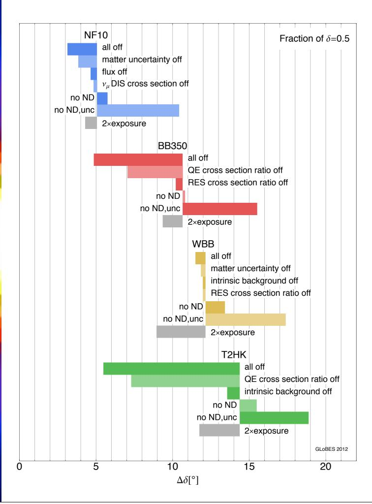
Good energy resolution, wide band beam, additional input will help in reducing the impact of systematic errors. The near detector(s) will play an important role.
