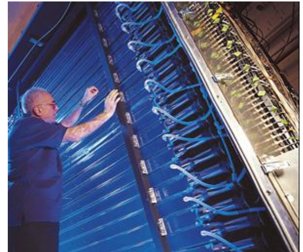
Michigan University: 'neutron wall'. The flat-sided glass tubes contain liquid scintillator.
