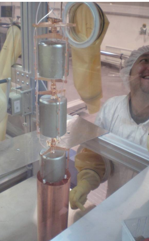
65µm Cu cylinder ('mini-shroud') to shield E-field
