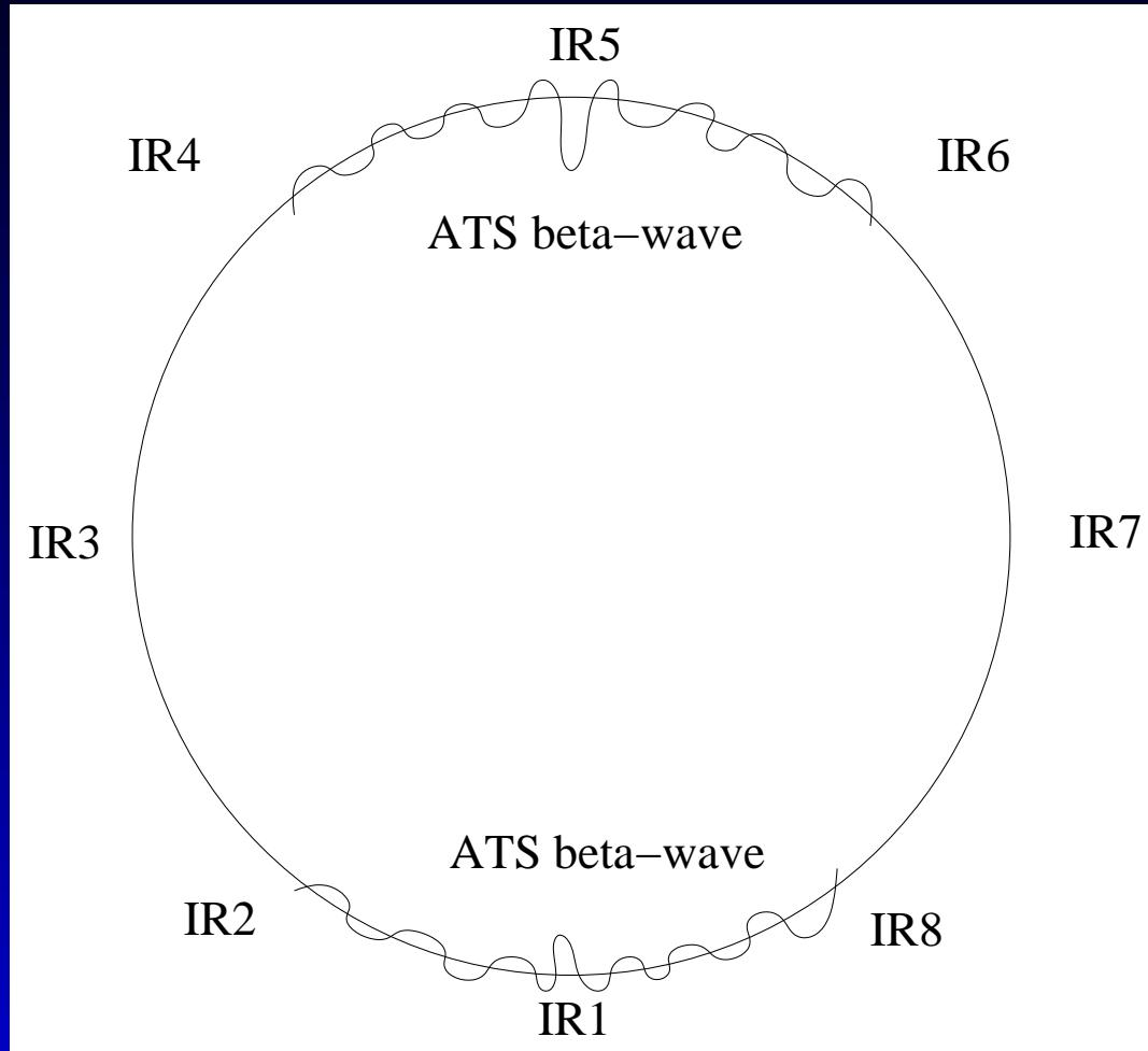
ATS optics uses IR2 quadrupoles to squeeze  $\beta^*$  in IR1.
