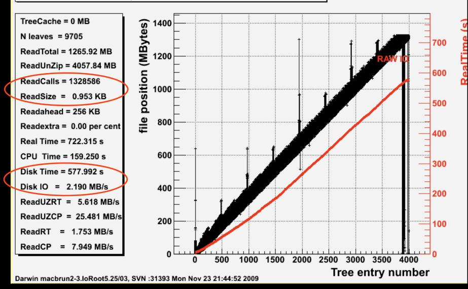
Performance measurements made using the TTreePerfStats class
