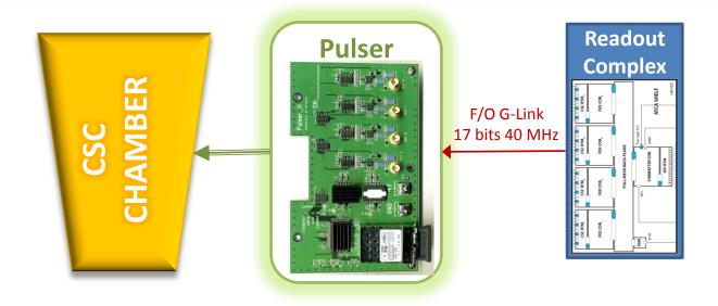
The Pulser provides a fast voltage step to the calibration planes of the on-detector electronics channels simulating a particle interacting with the Cathode Strips of the CSC. Control is externally delivered via the fiber optic link.
