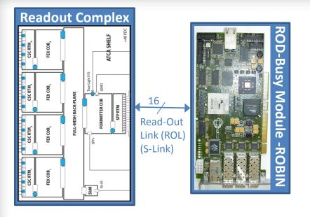
A **Read-Out Subsystem** has as many as 12 Read-Out Links (ROL), implemented as a Simple Link (S-Link). Each link's bandwidth is 160 MBytes/second. Includes XON/XOFF as the data flow control mechanism. The CSC event data is transmitted over 16 ROLs.
