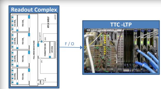
The **TTC-LTP** provides the ROD Complex with all the trigger and timing signals originated from the CTP (BC clock, L1A, BCID, EVID, reset, trigger type, etc.).
