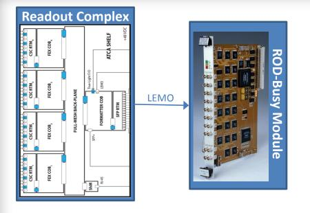
The **ROD-Busy Module** receives the BUSY signal from the detector and relays it to the CTP, thus inhibiting and throttling the L1A rate. This module also monitors and controls the busy levels during the run (stop-less removal).
