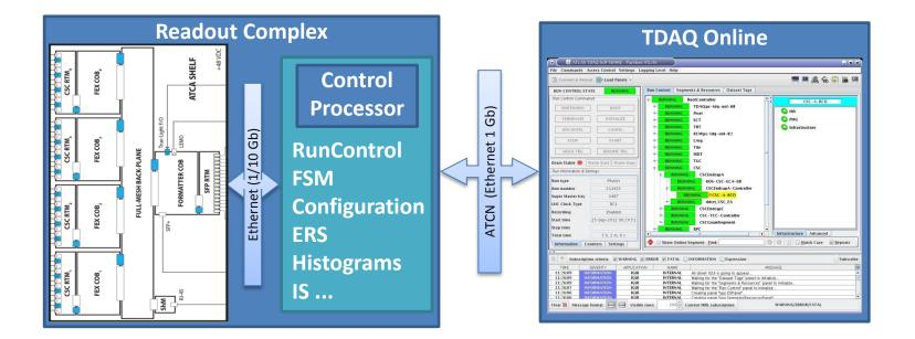
Some of the TDAQ software packages are essential to integrate the CSC with the TDAQ infrastructure. For example a RunControl application will be present to control and configure the ROD Complex. Other packages are required for monitoring purposes. The TDAQ release is installed in the network file system in P1.
