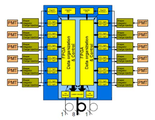
Scheme for 12-PMT MainBoard
