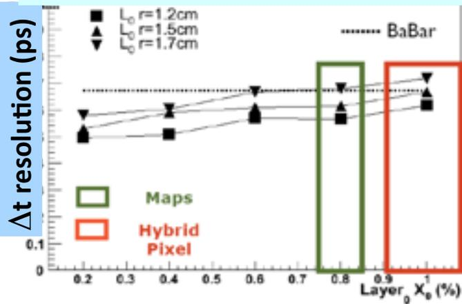
Layer0 technology can impact the per-event error on  $S$  by up to 12% (25% more luminosity needed to reach a given sensitivity)
