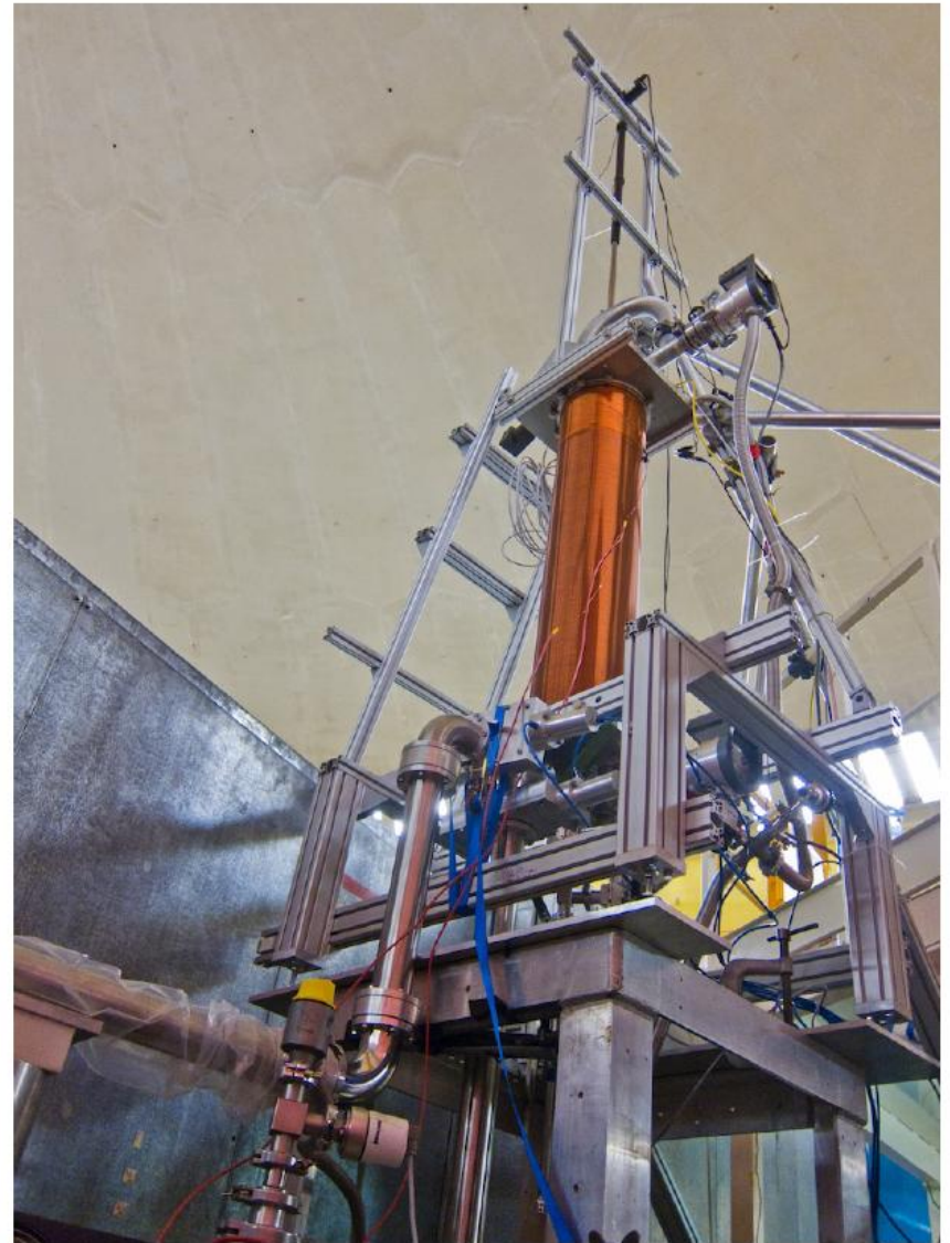
Storage time constant of trap closed with teflon plug: 800 s (PhD thesis Kent Leung)
