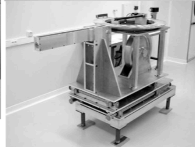
"Carousel" brick dispensing and storage system
