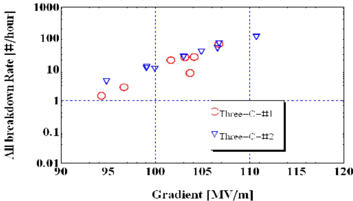
The near perfect surface processing affected only the processing time. The second structure processed to maximum gradient in a few minutes vs few hours for the normally processed structure.
