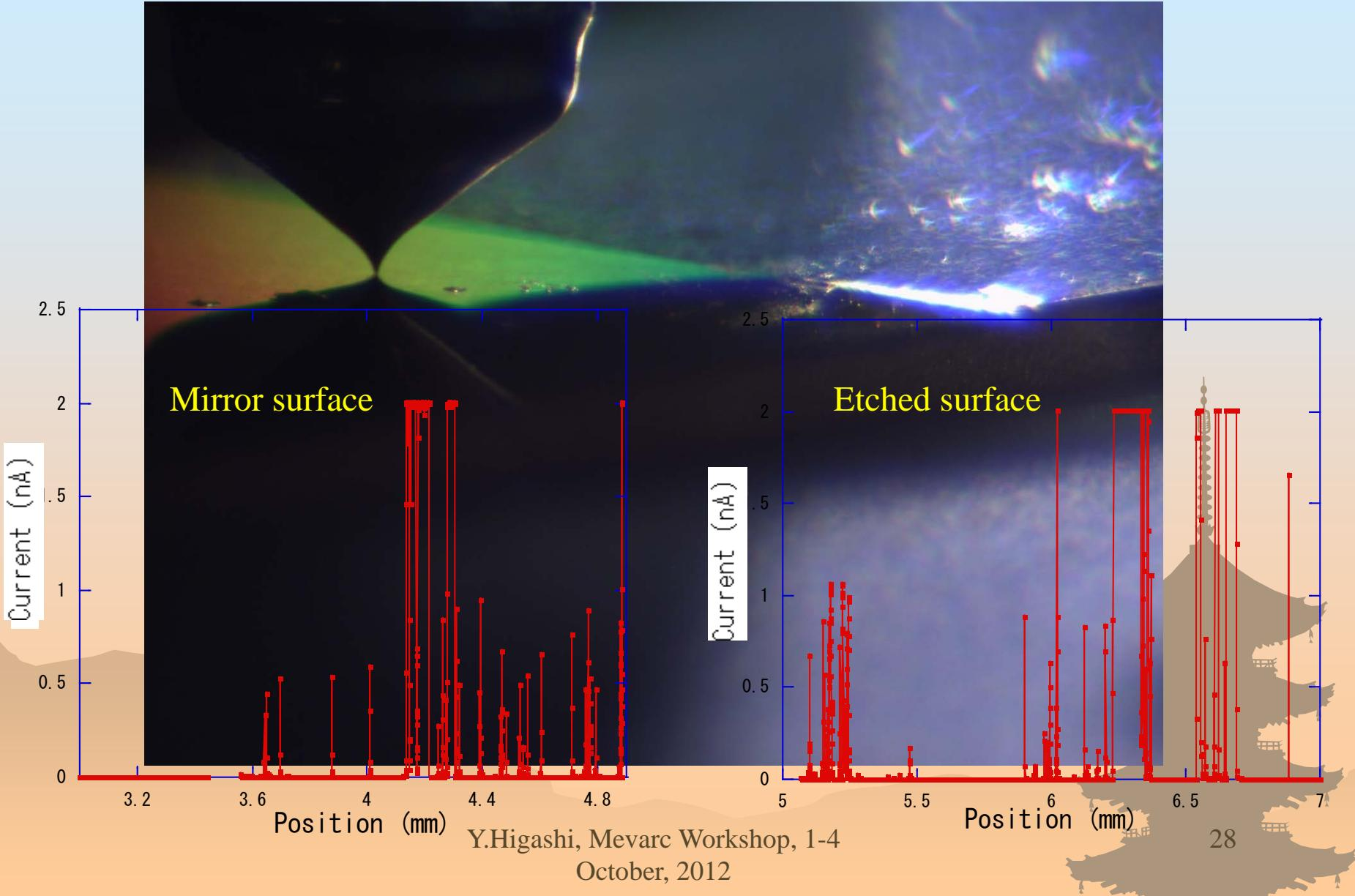
We found no surface damages after scanning on mirror surface
