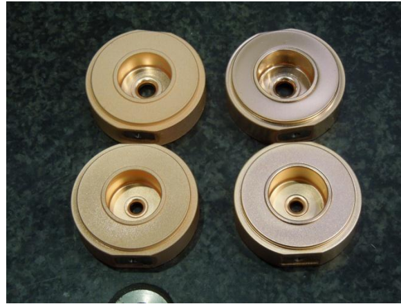
Stainless steel base plated with copper
