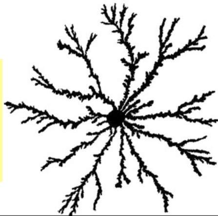
dendritic copper sulfate growth by electro-deposition
