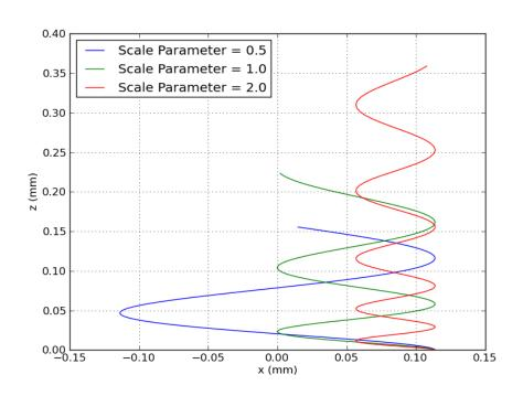
Gyro-radius scales inversely with scaling parameter demonstrating proper scaling for magnetic field
