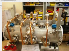
Assembly of the tank and RF network.
