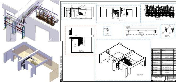
← 3D Model and 2D drawings for the layout of cooling water system for thermal test of TM0 in lab. (completed)
