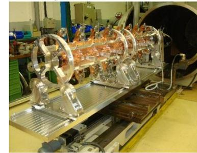
↑ Preparation of lifting / handling sequence of AS Assembly for EBW. (completed)
