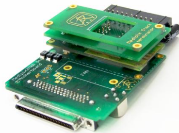
Prototype of the fast neutron detector. Stackable structure allows to add more layers.
