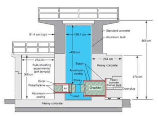
Reactor: 250 kW maximum power, can be regulated to few W. Total flux at maximum power is  $4x10^{12}$  cm<sup>-2</sup>s<sup>-1</sup> (central channel). NIEL (in Si) damage constant is 0.9 for fast neutrons. Several in-core and ex-core irradiation channels Maximum uninterrupted irradiation time is 16h. Highest fluence for AIDA  $10^{17}$  cm<sup>-2</sup> All irradiations done in two irradiation tubes. Accuracy of fluence is  $\pm$  10%
