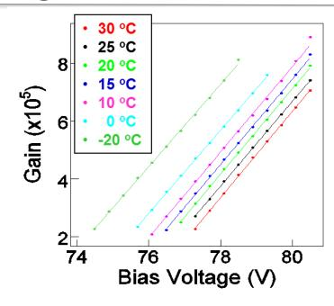
← linear dependence for breakdown V
