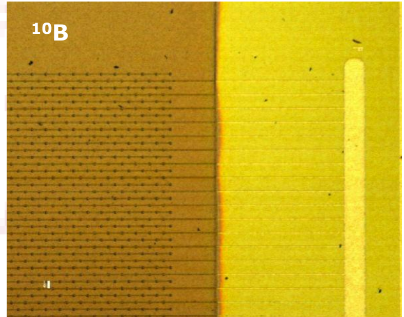
Prototype sensor with ^{10}\text{B} layer
