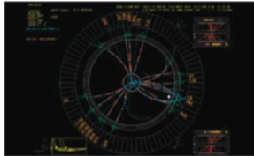
A simulated event in the JADE detector, generated using a refined Monte Carlo program and reconstructed using revitalized software more than 10 years after the end of the experiment. (Courtesy Sigi Bethke.)
