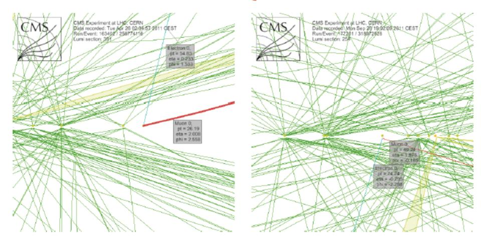
Figure 45: Event displays of the two events passing all selection criteria with  $p_T(\mu^{\pm}e^{\mp}) > 30$  GeV.
