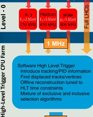
Software High Level Trigger Introduce tracking/PID information Find displaced tracks/vertices Offline reconstruction tuned to **HLT** time constraints Mixture of exclusive and inclusive selection algorithms
