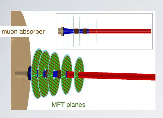
5 circular Si-pixel planes covering (most of) muon arm acceptance:  $-3.6 < \eta < -2.5$
