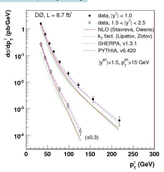
$$\frac{d\sigma}{dp_T^{\gamma}} = \frac{N_{evt} \times f_{\gamma} \times f_b}{A \times \varepsilon \times L \times \Delta p_T^{\gamma}}$$
