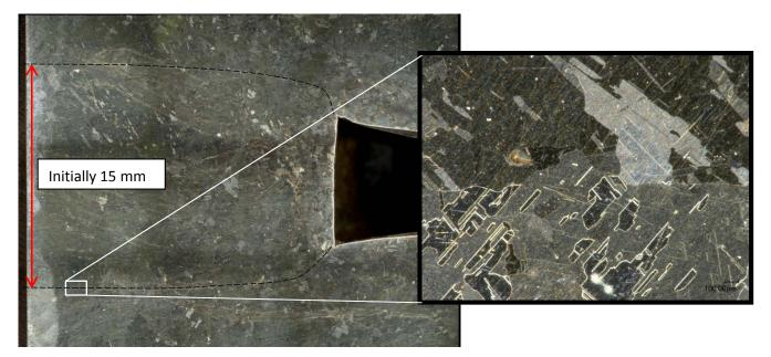
Even with 10 MPa bonding quality is good, but severe plastic deformation
