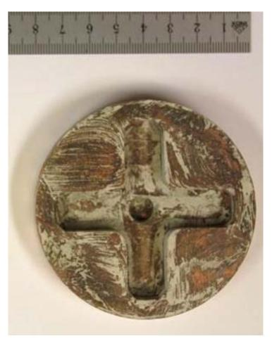
Zinc oxide paste helped keeping copper not being attached to the stainless steel surfaces
