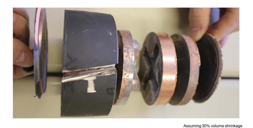
"succesful" dismantlement (major difficulties in order to remove the thick capsule ring; only possible after stress release cutting -> destroyed)
