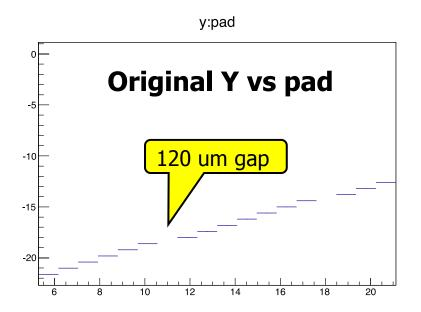
This particular TPC row seems to be miscalibrated to 140um -> accuracy of the Fast Transformation [80um] here is not worse than the accuracy of the original transformation [140um].
