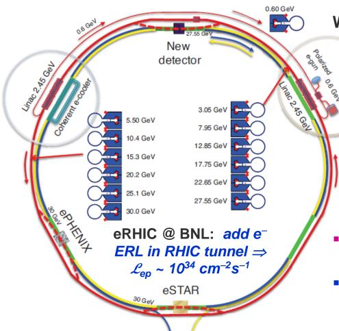
Design allows easy staging (start w/ 5-10 GeV, upgrade to ~20 GeV e<sup>-</sup>). Underwent successful technical design review in 2011. Bottom-up cost eval. + value engineering in progress.
