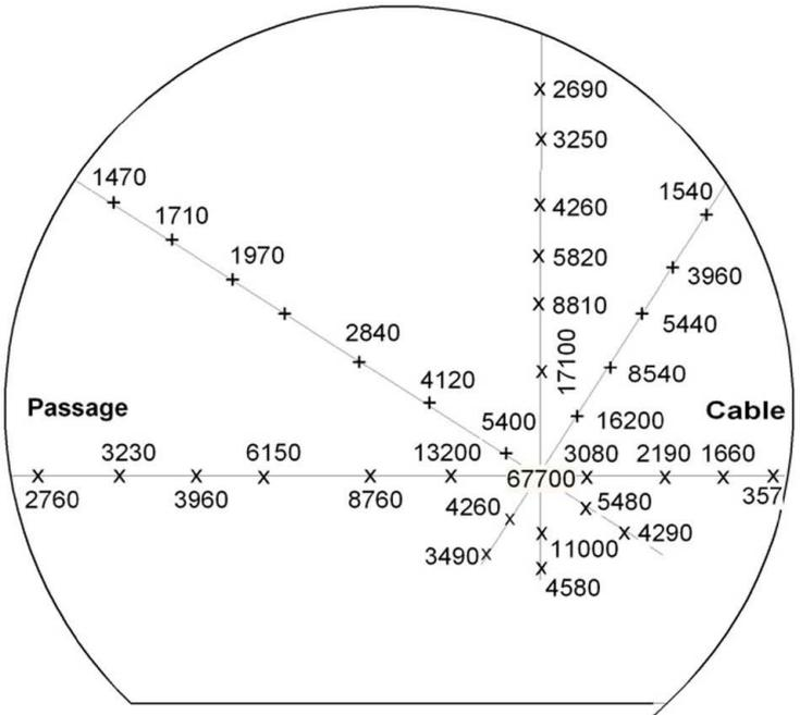
Cross-section 1 in the arc 11.55 m from the RF chicane
