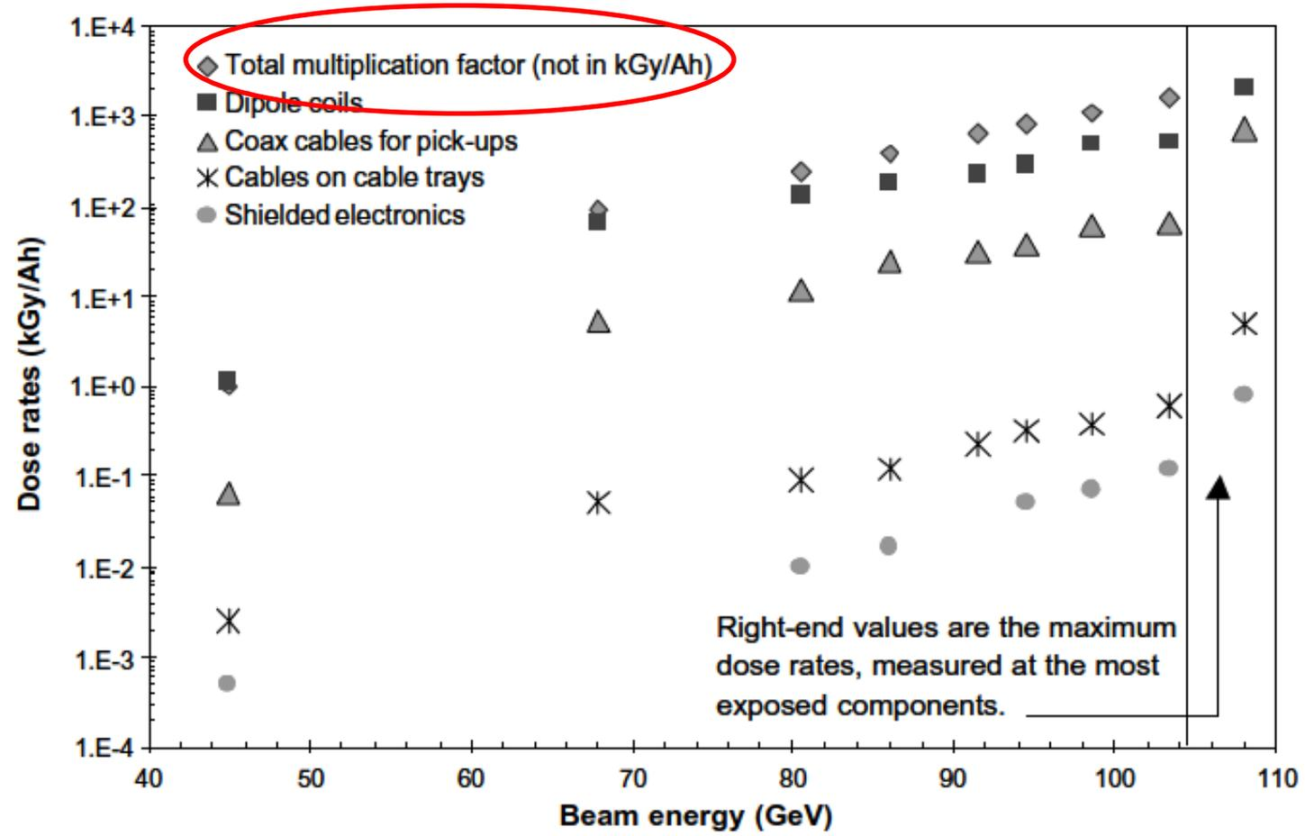
Evolution of the dose rates (kGy/Ah) in the arcs as a function of the beam energy (GeV)
