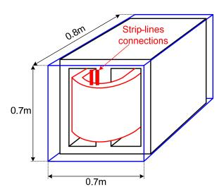
The strip-lines connections can be easily placed on the 0.7mx0.7m face (either the front or the back one of the Figure). The primary connections would be on one of these two faces as well. The strip line size will have 1000mm<sup>2</sup> of cross-section. Transformers will be relatively easily stackable. The weight of each transformer is estimated between 350kg and 450kg.
