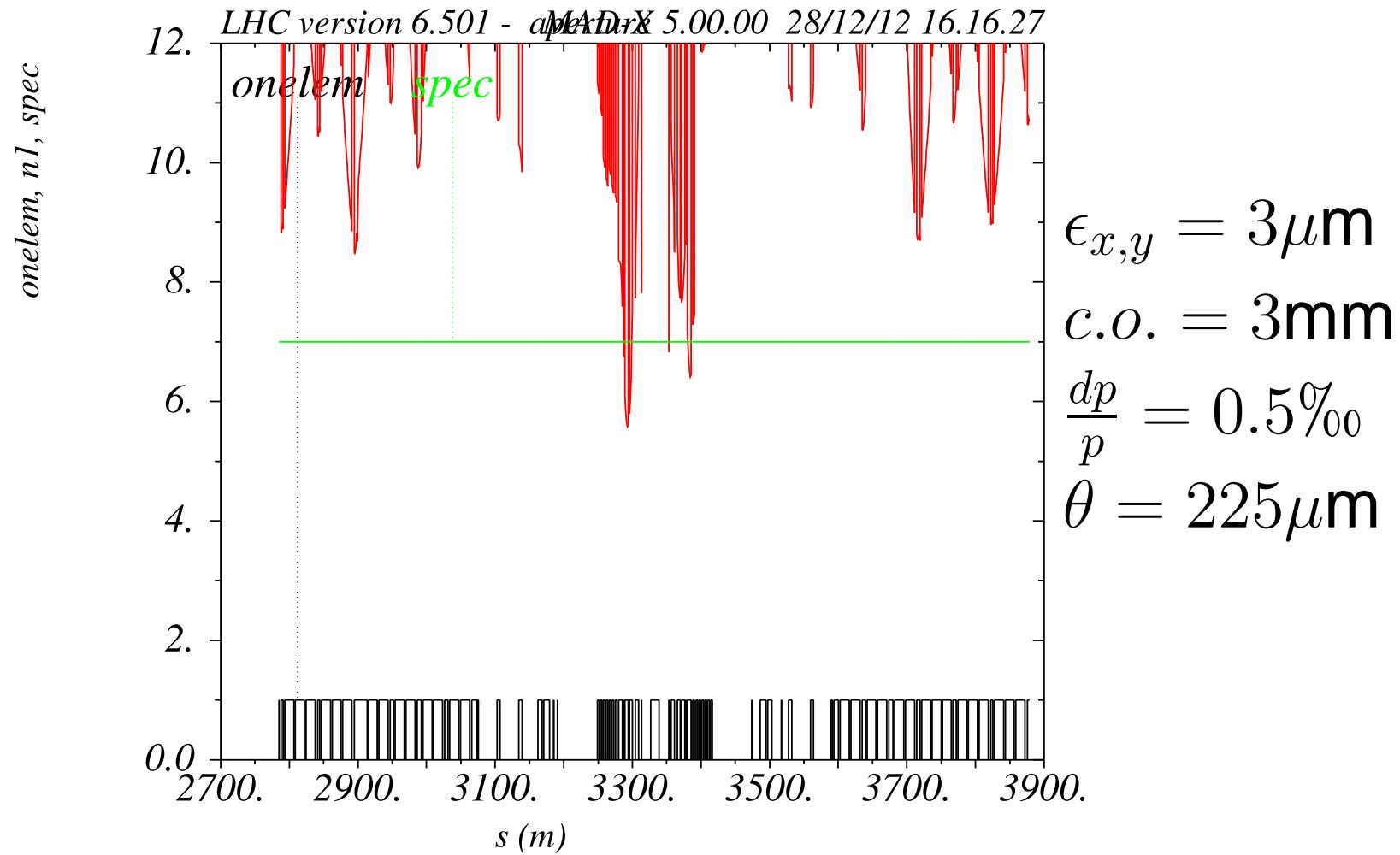
Aperture not OK at  $\beta^* \geq 5$  m.
