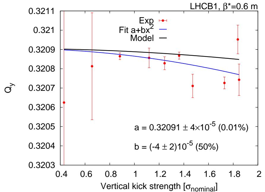
Lower excitation amplitude and poorer amplitude detuning measurement, yet consistent with model.
