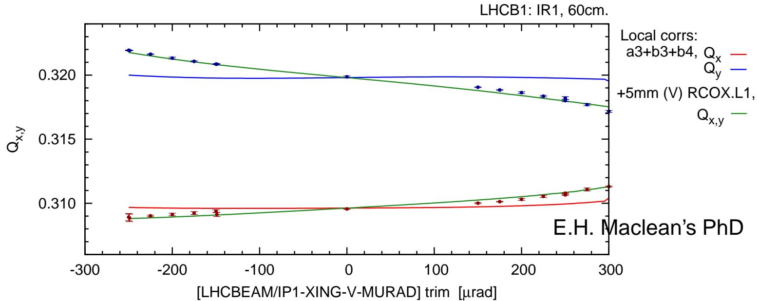
A vertical misalignment of  $\approx 5\text{mm}$  in RCOX.L1 explains the observation. This should be carefully taken into account in future IR corrections.
