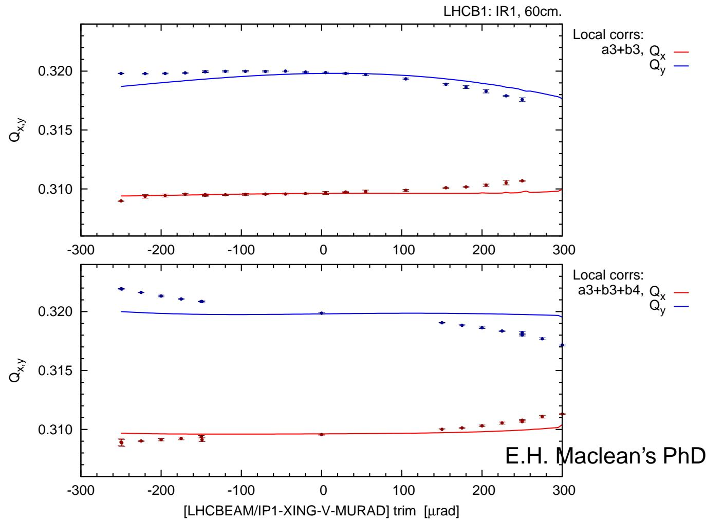
a3 and b3 corrections OK. Large discrepancy when applying the b4 correction.
