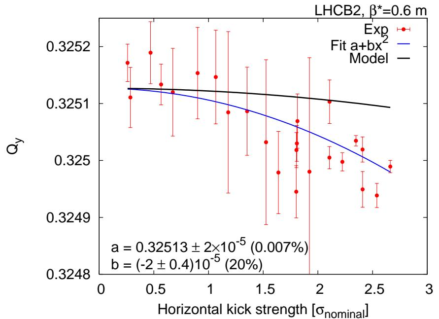
First measurement of amplitude detuning with AC dipoles! IR1 and IR5 corrections are in. AC dipole effect on model is under investigation.
