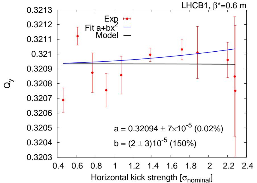
Beam 1 seems to have smaller amplitude detuning than Beam 2. Measurement still poor and consistent with model.
