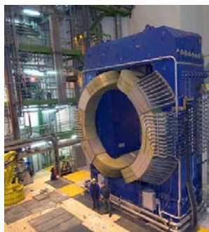
Fig 2: ALICE spectrometer dipole
