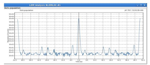
With 25 ns beams we have to go back to main-main collisions, the interest will then shift back to satellites at injection and luminosity calibration runs.
