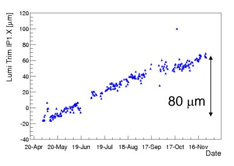
Orbit correction at IP to bring beams head-on (here B1H correction).
