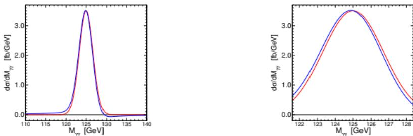
$M_{\gamma\gamma}$  resolution: Gaussian ( $\sigma_M = 1.7 \text{ GeV}$ ),  $H \rightarrow \gamma\gamma$  peak shift:  $\mathcal{O}(-150 \text{ MeV})$
