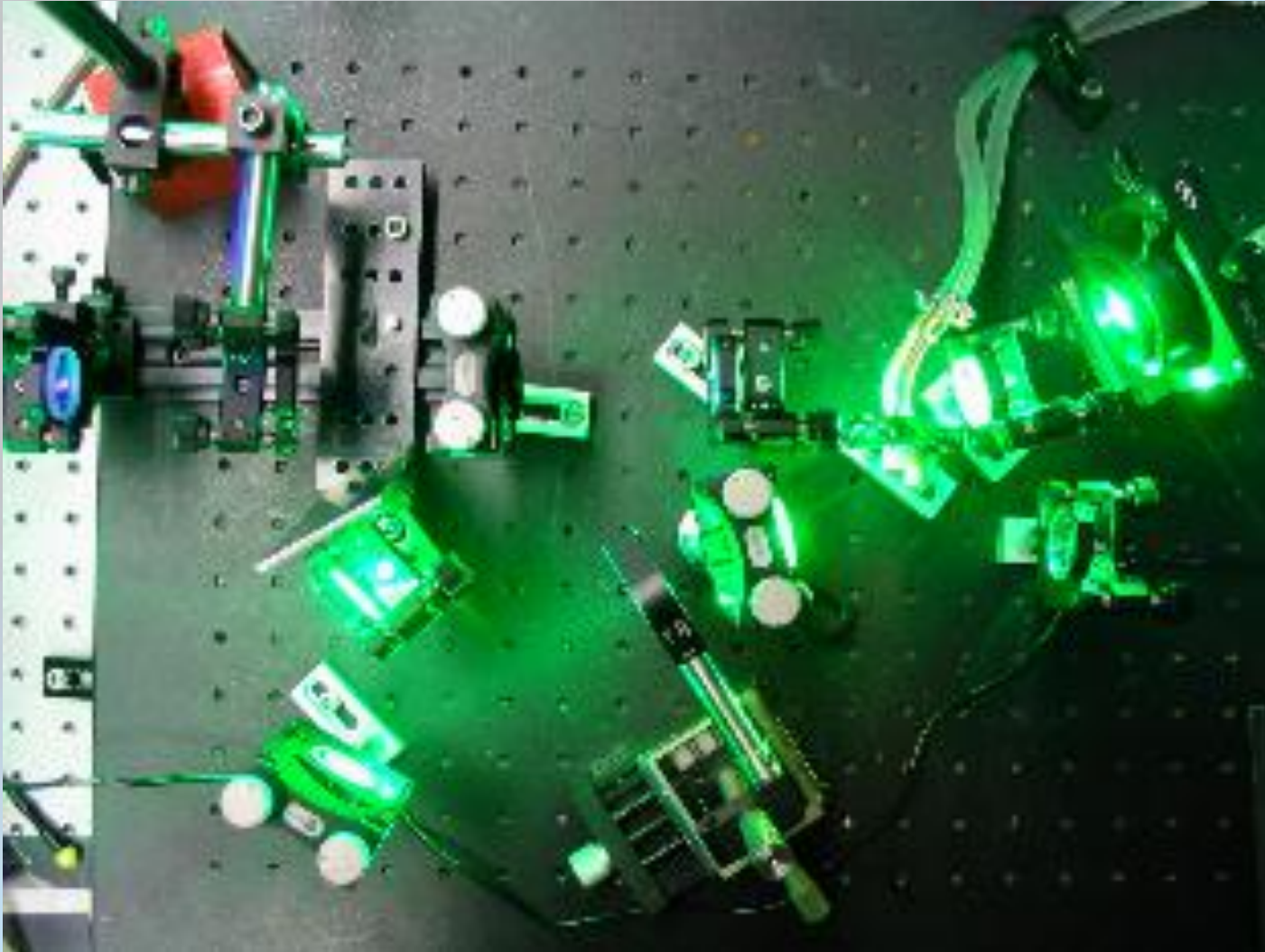
Intra-cavity SHG, T.Kessler (DPG 2004)
