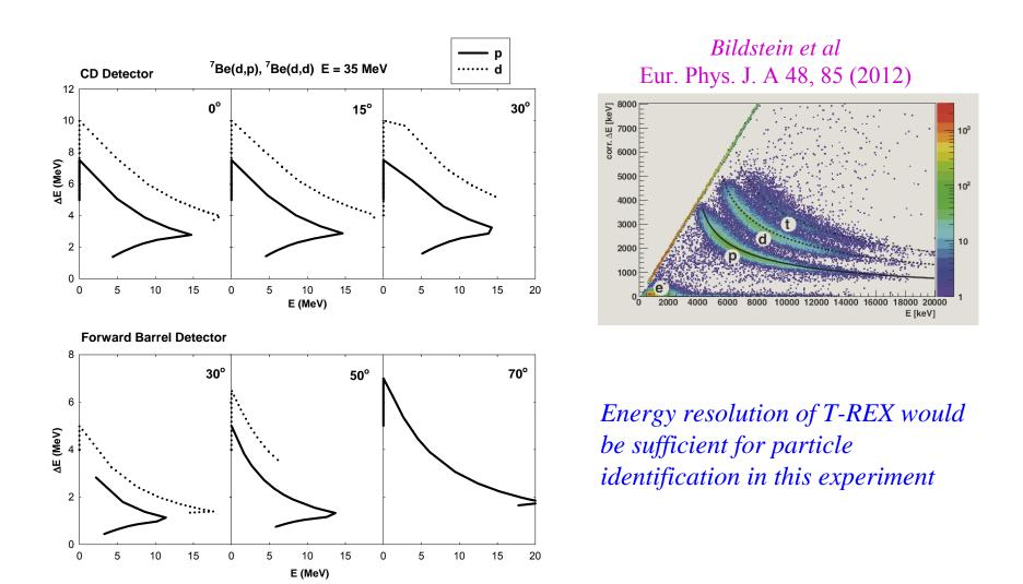
Excitation energies of the populated states of interest can be reconstructed from deposited energies in various detectors for stopping particles. Breakup of  $^8\text{Be} \to 2\alpha$  particles that stop in  $\Delta E$  detectors of T-REX, can be identified by using a multiplicity trigger.
