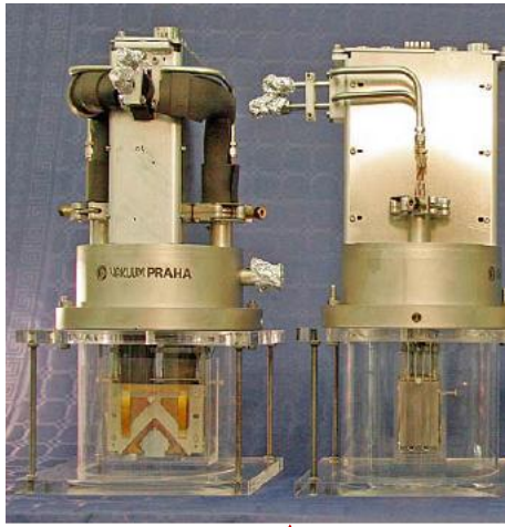
Separation of high LHC vacuum from detector vacuum
