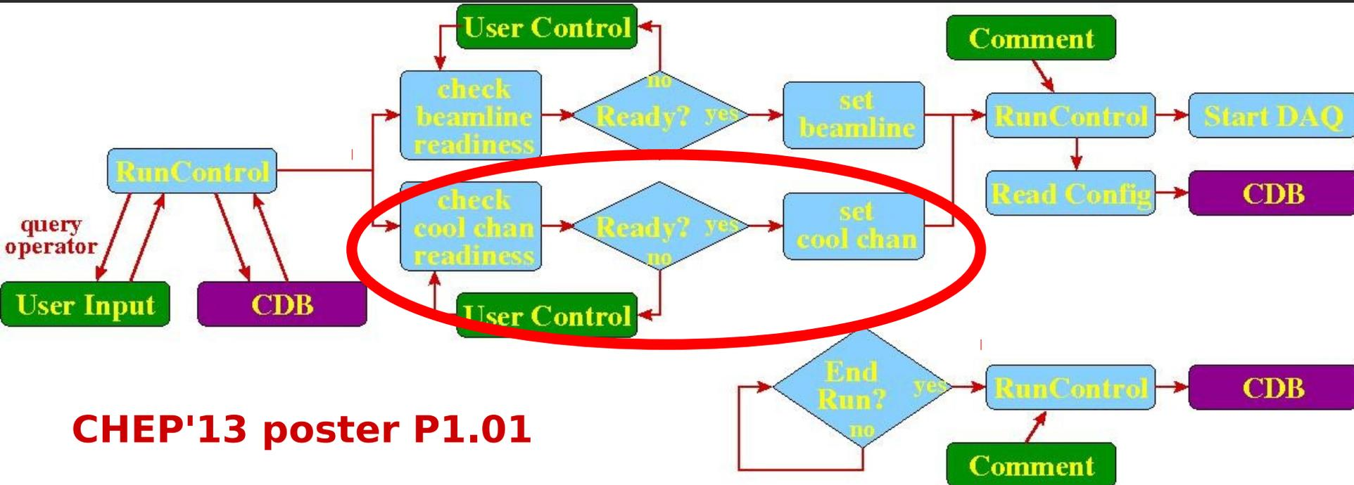
State machines for magnet control greatly reduces complexity of RunControl. RC need only check state of each magnet.
