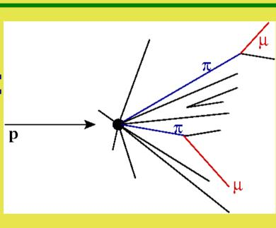
Created with large emittance (6D volume/momentum) spread) - impractical for an accelerator. "Cooling" reduces beam spread. Short muon lifetime,  $\tau_{\mu}$ =2.2 $\mu$ s, dictates ionization cooling as only feasible technique.
