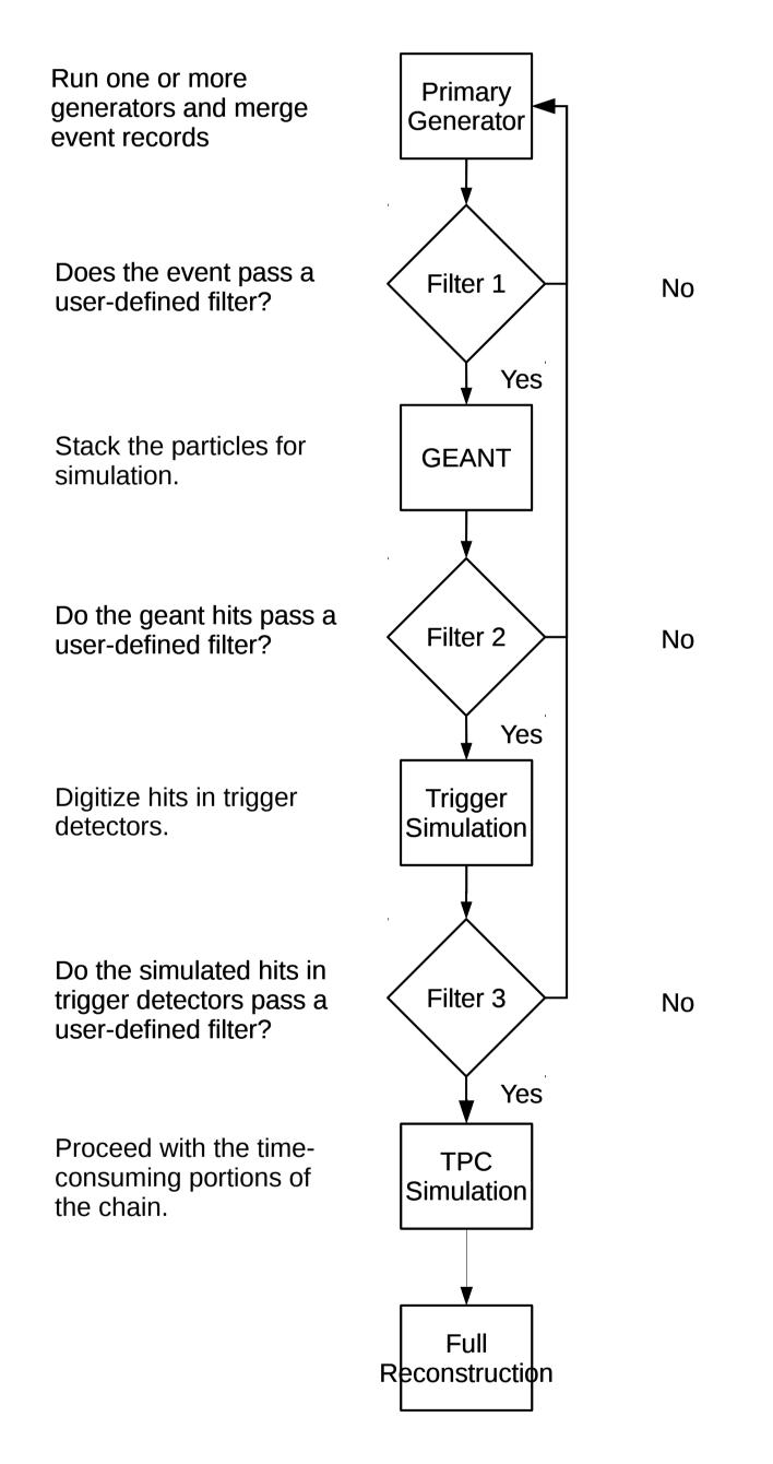
The STAR Primary Event generator is responsible for running the concrete event generators and assembling the event record. The event is passed to GEANT for full simulation, if it satisfies appropriate filter conditions.
