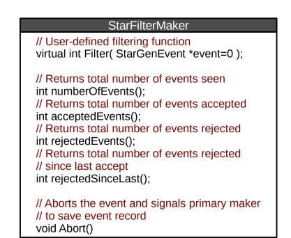
Filtering enables us to examine the generated event at an early stage in the simulation, and stop processing it if it is unlikely to be of use in offline analysis. This saves us from passing unnecessary events to the more computationally demanding parts of the simulation chain.
