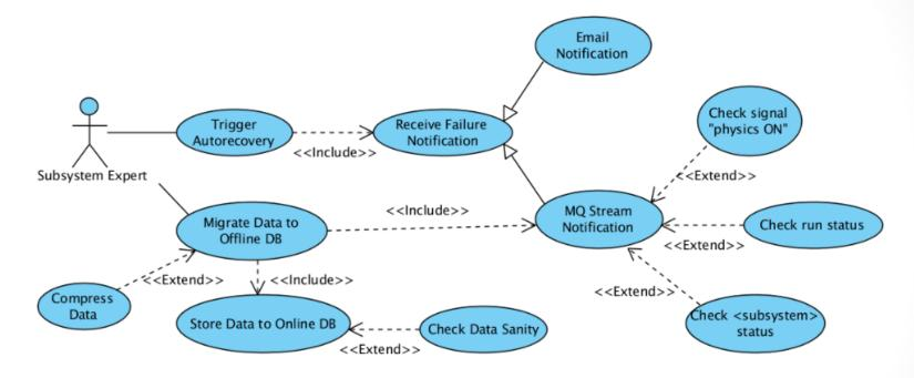
STAR Subsystem services located in online domain depend on other subsystem states including Trigger, DAQ and the data exported from collider run-time systems..
