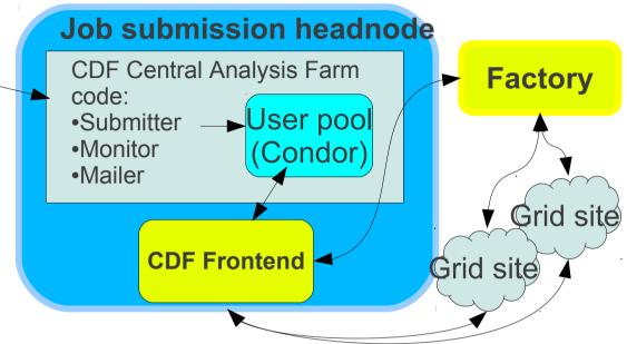
Based on *glideinWMS* workload management system (batch system = *Condor*)
