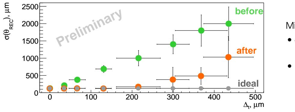
Misalignment of: • 50  $\mu$ m already disturbs reconstruction • up to 250  $\mu$ m can be corrected Expected mechanical accuracy ( $\Delta_{trans} \sim$  200  $\mu$ m,  $\Delta_{rot} \sim$  3mrad )
