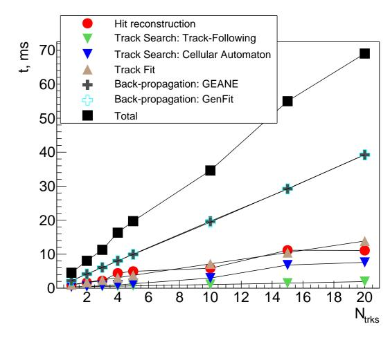
slowest process  $\rightarrow$  Back Propagation fastest process  $\rightarrow$  Track Following
