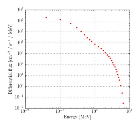
Differential flux (SPENVIS/AP-8 trapped electron model).
