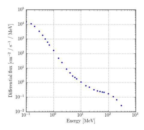
Differential flux (SPENVIS/AP-8 trapped proton model).
