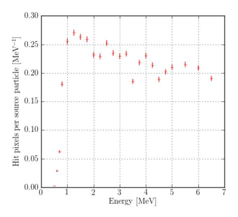
Hit pixels per source particle (SimLucid GEANT4 model).
