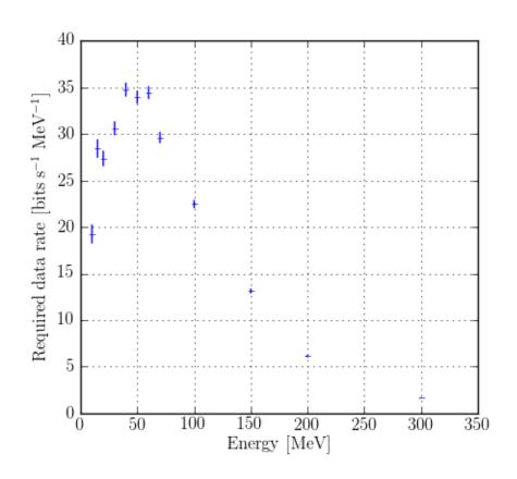
Required data rate summed over all energy bins due to trapped protons in LEO:
