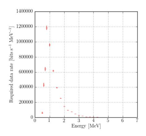
Required data rate summed over all energy bins due to trapped electrons in LEO:
