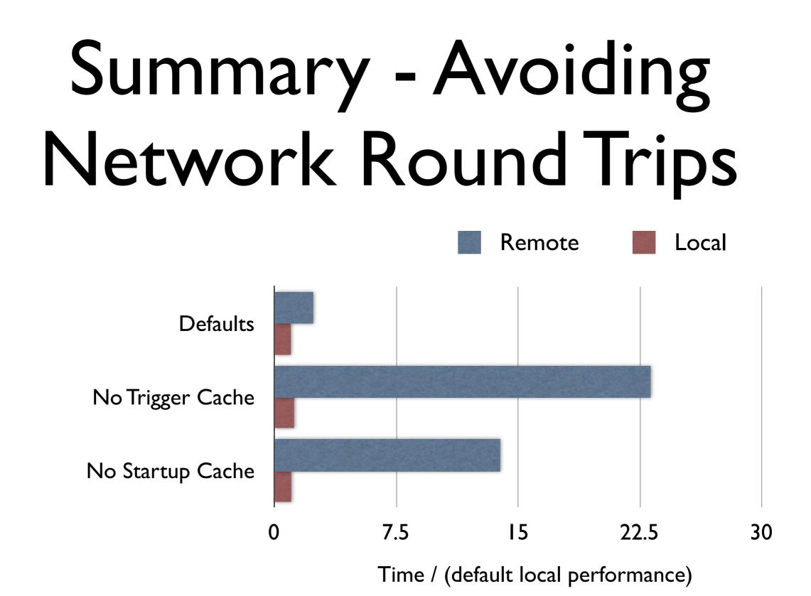
Not shown: ROOT defaults (no TTreeCache) reading remotely is 177x slower than CMSSW's defaults reading locally!
